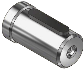
SHAFT B Cylindrical Shaft \varnothing 32 Parallel Key 10x8x45 METRIC
